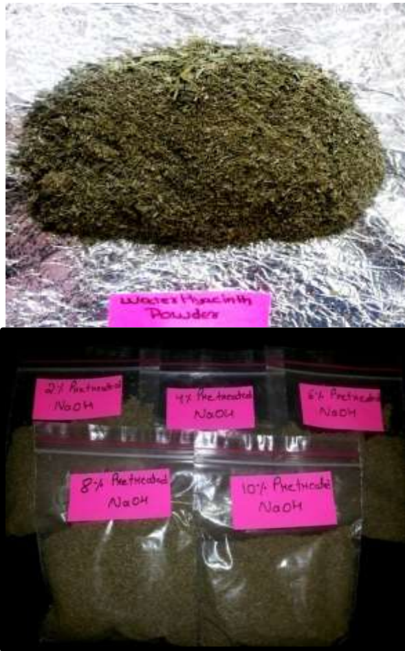
Fig 1: (a) Water hyacinth (leaves powder) (b) Water Hyacinth powder treated with different conc. of NaOH
